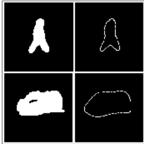
Figure 3. Example human and vehicle shapes and reconstructed boundaries using 10 FDs.
