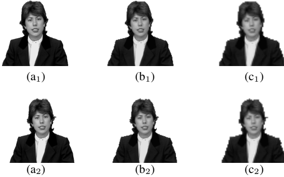
Fig. 3. Claire object of 23th frame; (a 1 ) scalable 288 \times 352 ; (b 1 ) scalable 144 \times 176 ; (c 1 ) scalable 72 \times 88 ; (a 2 ) regular 288 \times 352 ; (b 2 ) regular 144 \times 176 ; (c 2 ) regular 72 \times 88 ;
