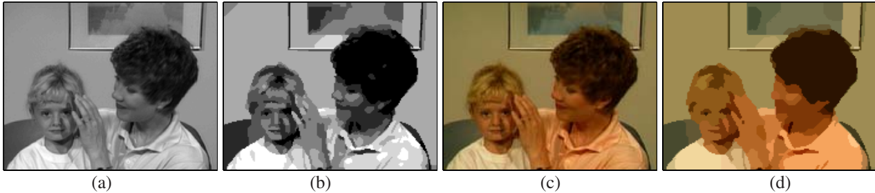
Fig. 5. Frame 34 of qcif size Mother and daughter Image sequence segmentation with \beta = 40 ; (a) original grey-level image; (b) regular grey-level single-resolution segmentation with k = 7 clusters; (c) color image where U and V are in half resolution; (d) Proposed scalable segmentation with k = 7, 2, 2 clusters.
