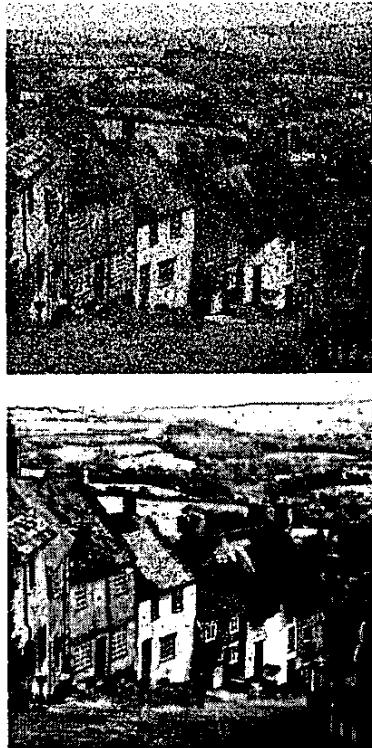
Fig. 4. Examples of decoded images where the original 8 bpp image was transmitted over a channel with an E_b/N_0 of 0 dB. Top: hard decoding; bottom: MS soft decoding.
