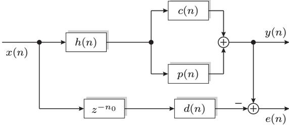
**Fig. 1.** Single-channel setup for room equalization.  $p(n)$  is a random perturbation of the assumed channel impulse response  $c(n)$ .
