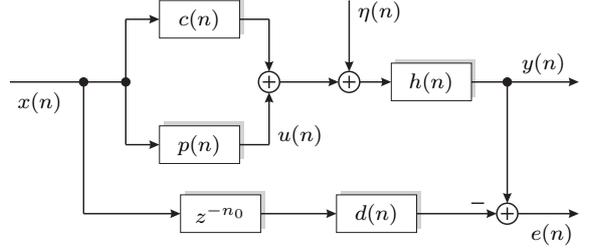
**Fig. 2.** Setup for memory truncation in data transmission.
