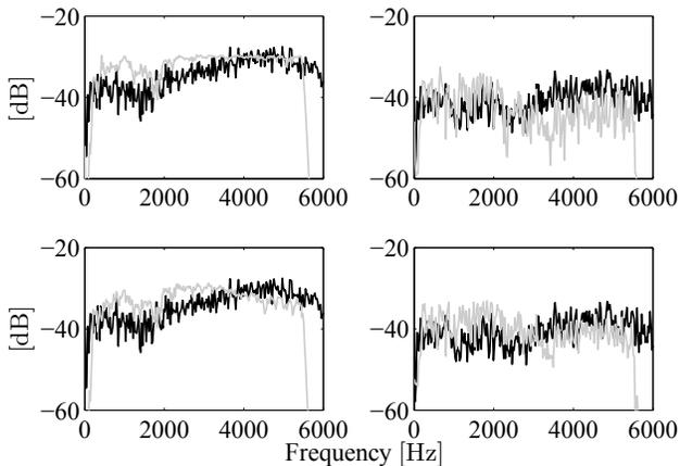
**Fig. 2.** Magnitude transfer functions (black) and processed magnitude transfer functions (gray). The upper left plot shows the ipsilateral path to the left ear and the upper right one the contralateral path to the left ear. For the upper plots we used a non-robust design and a robust design for the lower plots (again, ipsilateral path to the left ear on the lower left and contralateral path to the left ear on the lower right plot). The room impulse responses were not changed.
