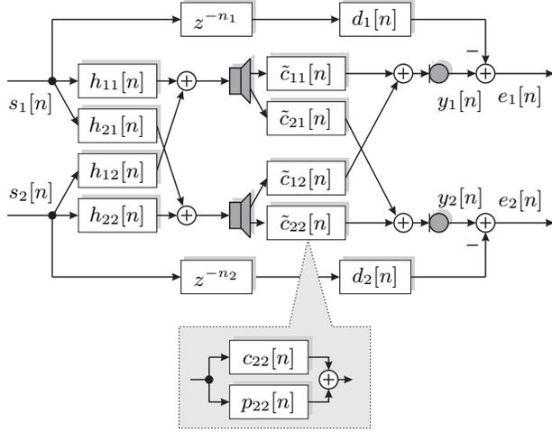
**Fig. 1.**  $2 \times 2$ -setup of a crosstalk canceller. For illustration purposes the generation of the error signals is also shown.
