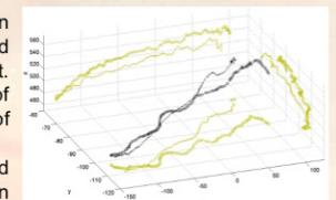
Precision of hand detection depends on the optical and geometrical setup and as well on the speed of the movement. In our case we reached a precision of approximately 8 mm<sup>3</sup> in a volume of about 50x40x20 cm<sup>3</sup> at 25 Hz. An exemplary 3D-trajectory of a hand movement can be seen in the figure on the right.
