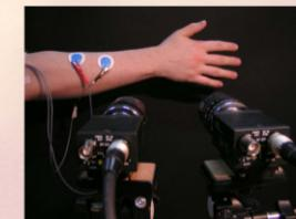
As proof of concept we recorded EMG signals (digital flexor muscle) correlated to a hand-grasp movement. The EMG signals of the volunteers main arm muscles were intercepted by self adhesive electrodes. The recordings are synchronized via high resolution system timestamps..
