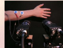
As proof of concept we recorded EMG signals (digital flexor muscle) correlated to a hand-grasp movement. The EMG signals of the volunteers main arm muscles were intercepted by self adhesive electrodes.
