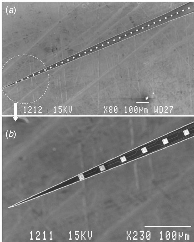
**Figure 4.** Scanning electron micrograph of (a) a silicon probe with 1 shaft  $\times$  32 electrodes and (b) close-up of a probe tip designed with  $4^\circ$  taper angle. The interconnect lines shown are  $1\ \mu\text{m}$  wide.
