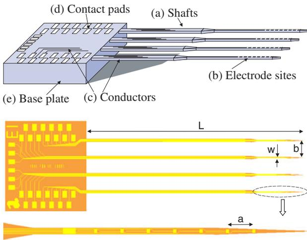
**Figure 1.** Schematic drawing of the probe structure described in the text (not to scale) and a typical CAD layout.
