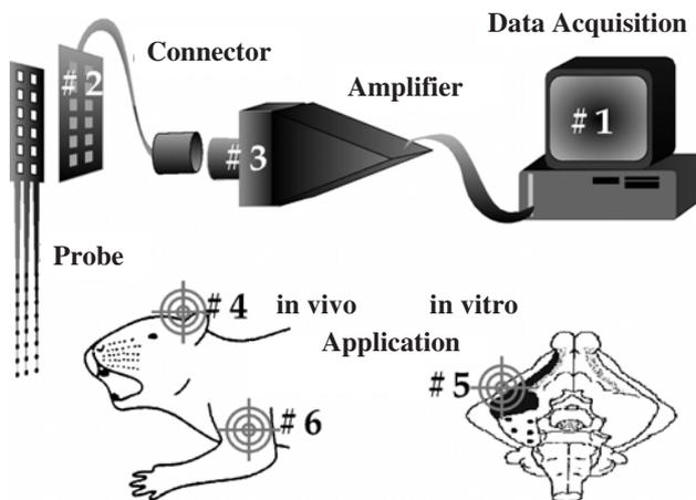
**Figure 7.** Overview of a complete recording system (1–3) and areas of application experiments (4–6) in the EU project VSAMUEL: 1. Data acquisition system, hardware and software; 2. custom designed connectors and batch fabricated multisite microelectrode probes; 3. discrete and modular multi-channel amplifier; 4. cerebellum; 5. cortex; 6. peripheral nerves.
