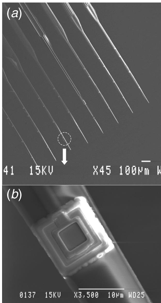
**Figure 3.** Scanning electron micrograph of (*a*) a silicon probe with 8 shafts  $\times$  4 electrodes and (*b*) close-up of a  $10\ \mu\text{m} \times 10\ \mu\text{m}$  Ir electrode site.
