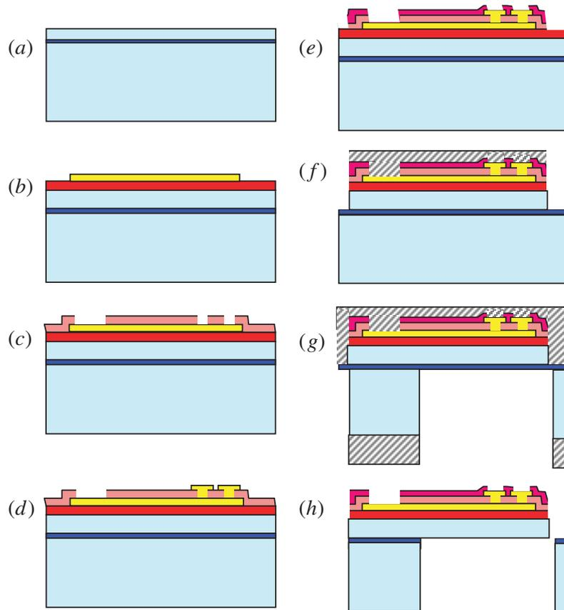
**Figure 2.** Schematic illustration of the fabrication process described in the text (not to scale). (a) SOI wafer, (b) SiN deposited, litho 1, Ti/Au deposited and lift off, (c) SiN deposited, litho 2 and nitride etch, (d) litho 3, Ti/Ir deposited and lift off, (e) SiN deposited, litho 4 and nitride etch, (f) litho 5, SiN etch and front side Si etch, (g) litho 6 and back side Si etch and (h) oxide etch and resist strip.
