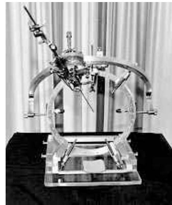
Fig.1: Riechert-Mundinger stereotactic frame ( www.neurosurgery.org/cybermuseum/stereotactichall/ )
