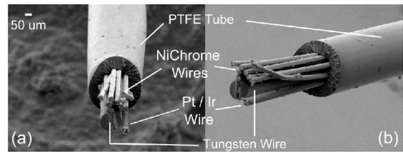
Fig. 5 : (a) & (b) An electron-micrograph of the Niotrode tip
