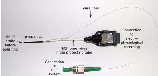
Fig. 7: An OCTrode assembly with its connectors
