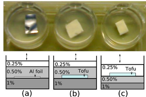
Fig. 6: The agar phantoms (a) with aluminum foil in the middle layer, (b) & (c) with tofu in the middle and top layers respectively
