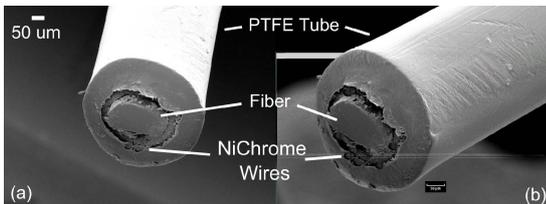
Fig. 9: REM micrographs of a typical OCTrode, covered with 30nm thick gold. The complete assembly’s diameter here is 255 $\mu$ m
