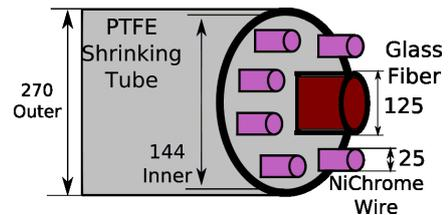
Fig. 1: Sketch of a multimodal multisite OCTrode. (All dimensions are in  $\mu\text{m}$ )
