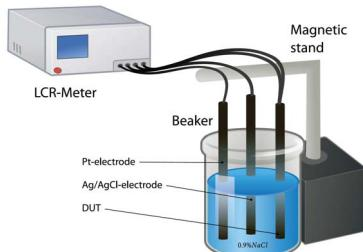
Fig. 4: Three point impedance measurement with counter, reference and working electrode immersed in electrolyte.
