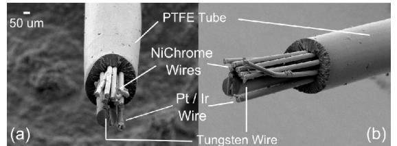
Fig. 5 : (a) & (b) An electron-micrograph of the Niotrode tip
