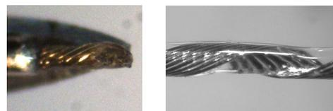
Fig. 2: original Niotrode (left) and original OCTrode (right).
