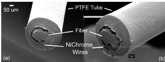
Fig. 9: REM micrographs of a typical OCTrode, covered with  $30\text{nm}$  thick gold. The complete assembly's diameter here is  $255\mu\text{m}$
