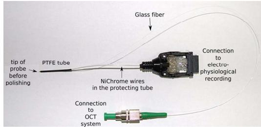
Fig. 7: An OCTrode assembly with its connectors
