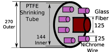
Fig. 1: Sketch of a multimodal multisite OCTrode. (All dimensions are in  $\mu$ m)
