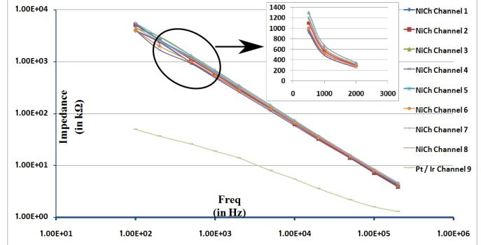
Fig. 10: Impedance of Niotrode microwires. Each of the nine wires was subsequently tested with the frequency range from  $100\text{ Hz} - 200\text{ kHz}$ .
