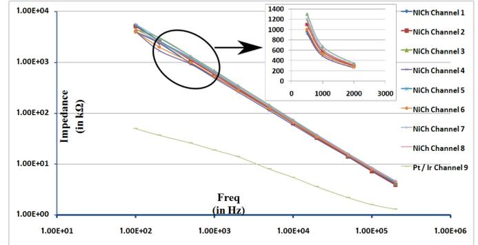
Fig. 10: Impedance of Niotrode microwires. Each of the nine wires was subsequently tested with the frequency range from 100 Hz – 200 kHz.
