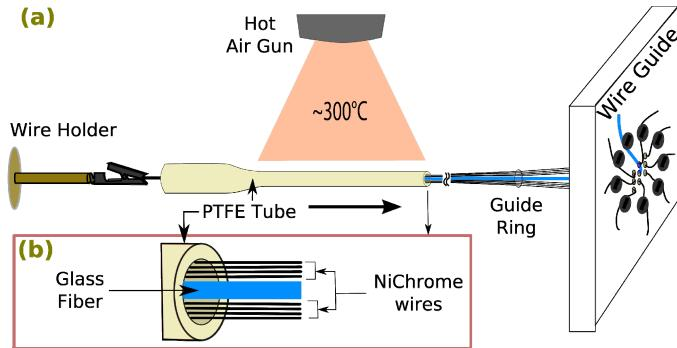
Fig. 3 : (a) A production setup of the OCTrodes (b) close view of the PTFE tube with inserted NiChrome wires and a monomode glass fiber
