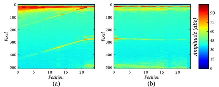
Fig. 11: The glass fiber was navigated in the agar phantom. (a) The aluminium foil is thus approaching towards the fiber tip. (b) The fiber can not penetrate the highly dense layer and loses the intensity due to bending at the tip.
