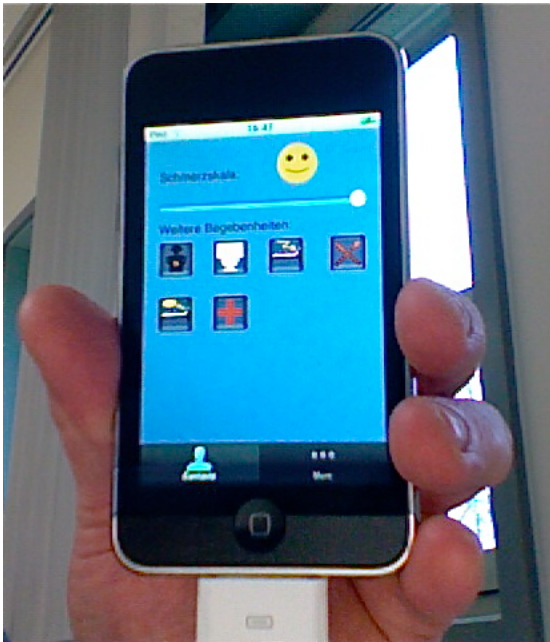
Fig. 2: iPain app running on an iPod touch . The upper trace with the visible „smiley“ is part of the NRS polling interface. Lower icons stand for links to input individual and time-stamped diary entrances.
