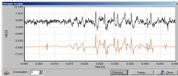
Fig. 11: Unfiltered (upper trace) and wavelet denoised signal (lower trace). The user can choose which type of denoising strategy and which wavelet he wishes to use. Here: Daubechies 2 and VisuShrink denoising.
