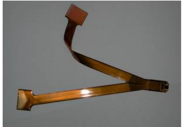
Fig. 4: Y-shaped flexible connector between microprobes (to be connected at the right side) and Molex ZIF connectors (to be connected left and top).
