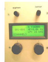
Fig. 6: Front panel user interface of PGMA-64. This interface allows gain settings of each of the 64 channels: either singly, in groups of 8, or all at once.
