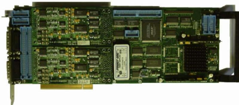
Figure 2: M67 DSP board equipped with two analog digital conversion modules
