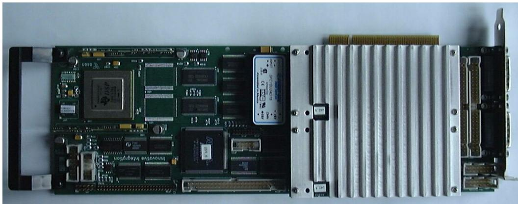
Figure 11: M67/Ad16 board equipped with heat spreader
