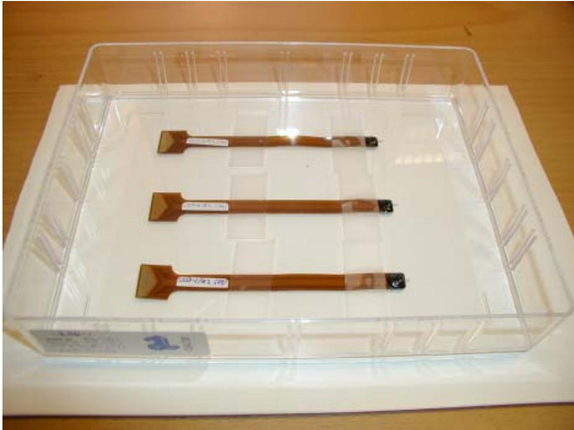
**Figure 3.7:** A set of probes ready to be delivered to a user group. The probe chips are mounted on flexible printed circuit substrates, wire-bonded, and glob-top protected.
