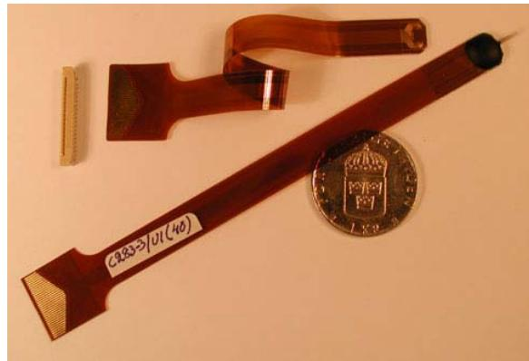
**Figure 5.** A neural probe chip mounted on a flexible printed circuit, wire-bonded and glob-top protected (right). A FPC without the glob-top cover is also shown (middle). The back end of the FPC was designed to mate with a 32-pin ZIF connector (shown left).
