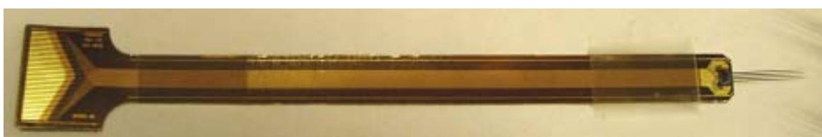
**Figure 3.6:** A silicon probe chip mounted on a flexible printed circuit. The left side of the printed circuit is designed to mate with the pre-amplifier of Work Package no. 3.
