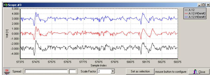
Figure 44: Denoising with db2 and db4 of a neural recording
