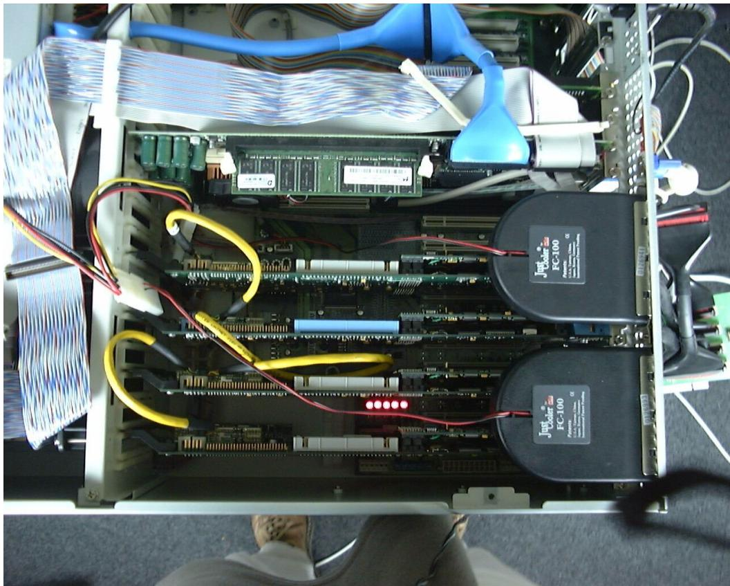
Figure 6: 128 channel data acquisition system (from top)
