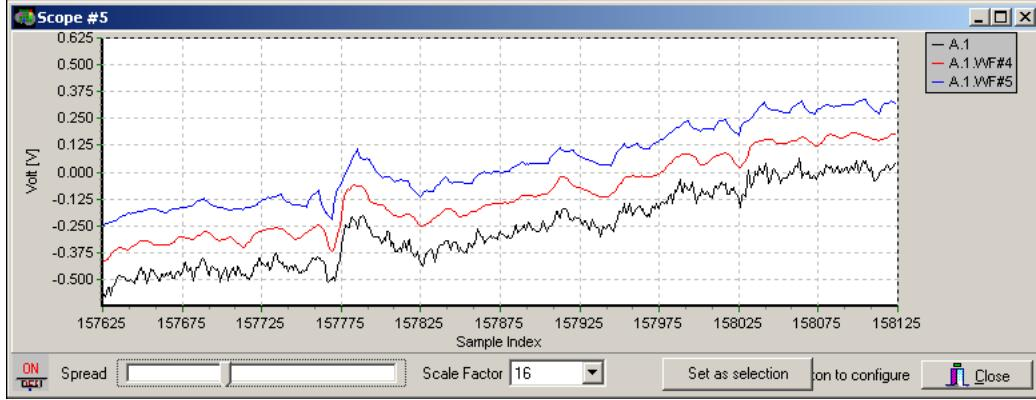
Figure 42: Low pass filter implemented with a wavelet filter bank. The lower black trace shows the original signal, the middle trace the db4 low pass filtered , and the upper trace the db2 low pass filtered version. The frequency bands 6.25-25kHz have been discarded.
