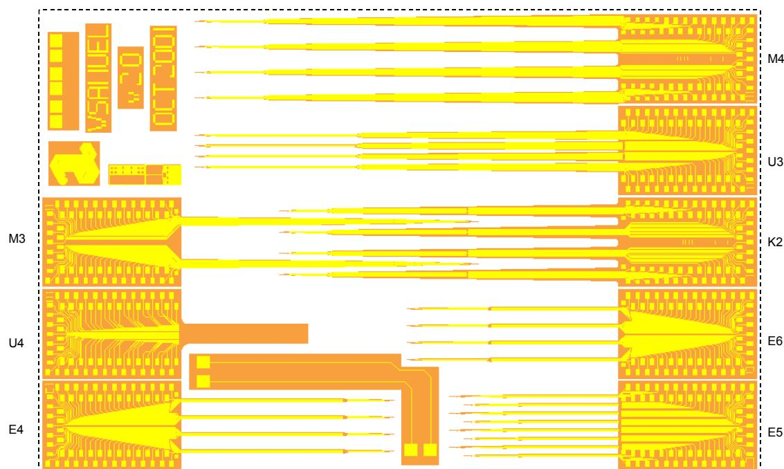
**Figure 2.2:** Stepper unit cell with eight 64-site probe designs.
