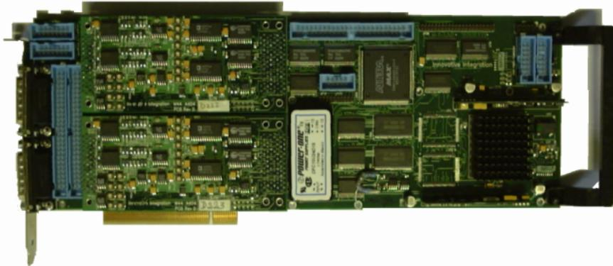
Figure 2: M67 DSP board equipped with two analog digital conversion modules
