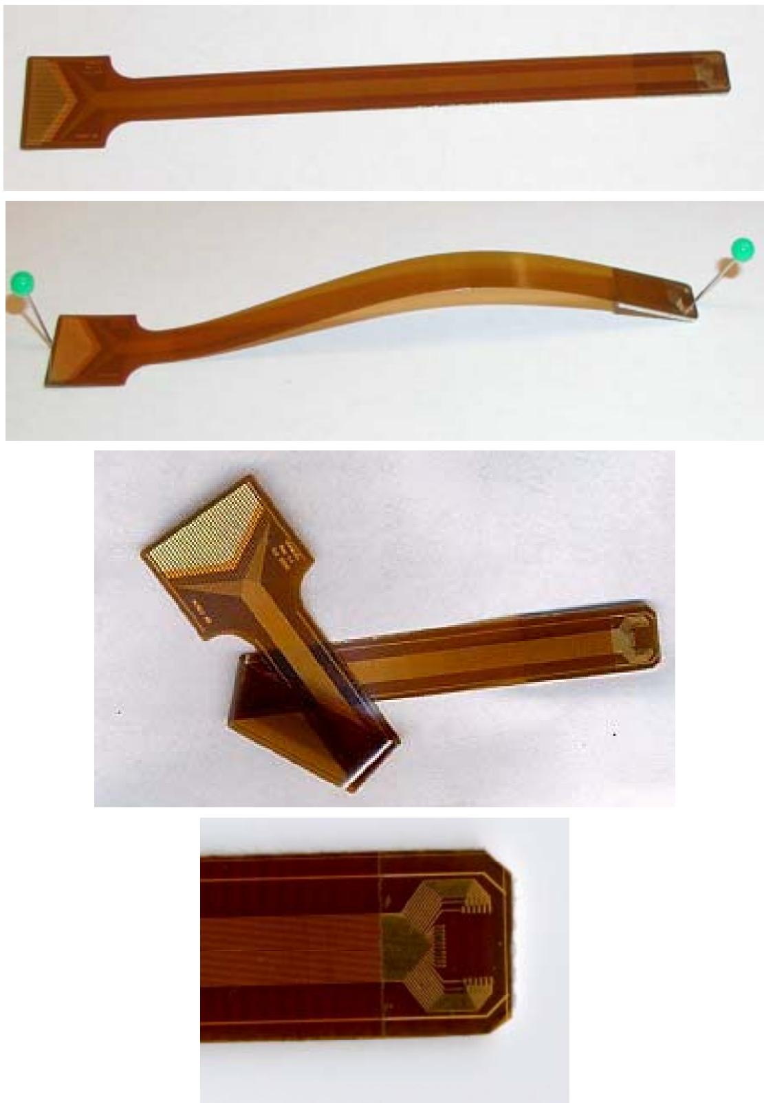
**Figure 3.1:** Flexible printed circuit manufactured by HP Etch (125.5 mm x 8.6 mm).
