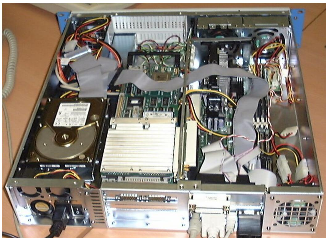
Figure 14: Small cabinet with improved air flow due to mulitple fans with M67/Ad16 board equipped with heat spreader
