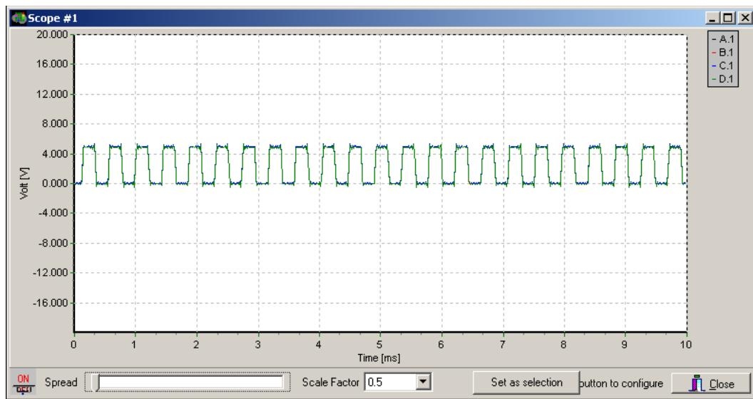
Figure 10: Overlay of the four channels in Figure 9 with spread set to zero
