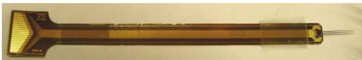
**Figure 4.1:** A silicon probe chip mounted on a FPC.
