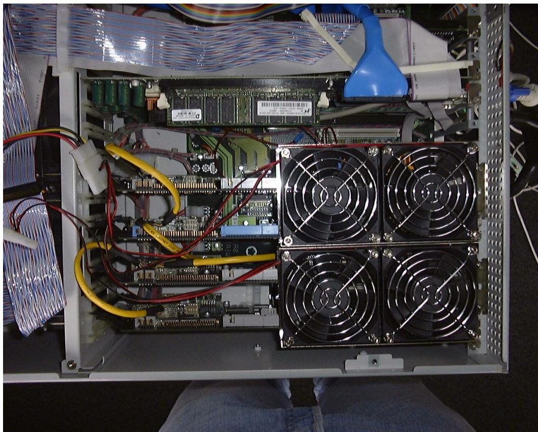
Figure 12: 128 channel data acquisition system prototype with additional fans
