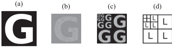
Fig. 3. Noise propagation through wavelet transform. (a) Noisemap (variance of 250 in white areas and 0 in black areas). (b) Single input image for wavelet transformation with Gaussian noise variance according to noisemap (a) and mean of 128. (c) Empirical noisemap in D4 wavelet space measured over 100 transformed input images. (d) Dyadic wavelet levels for noise propagation.
