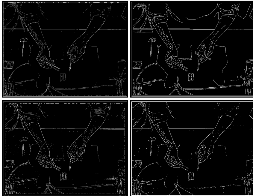
Fig. 3. Result of running edge detection on the top left frame from Fig. 5. Sobel edge detector with higher threshold – white edges – and lower threshold – gray edges – (top left). Canny edge detector (top right). Laplacian-of-Gaussian edge detector (bottom left). SUSAN edge detector (bottom right).
