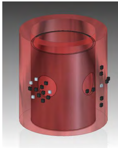
Figure 2. Artistic rendering of the two concentric beakers and a neoprene sleeve with circular windows around the inner beaker. Star (left) and plus (right) sensors are mounted centrally over of each of these windows.
