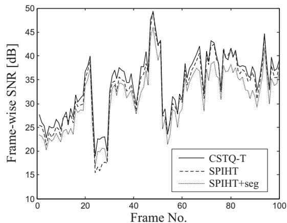
Fig. 2: Frame-wise SNRs for the first 100 frames of the svega signal, coded at 96 kbps.
