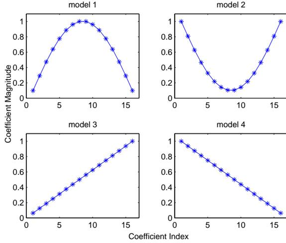
Fig. 1: Approximation magnitude distribution models (model 1,2: symmetric models; model 3: increasing model; model 4: decreasing model).
