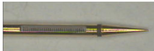
Figure 1: 31 electrodes linearly arranged on one shaft.
