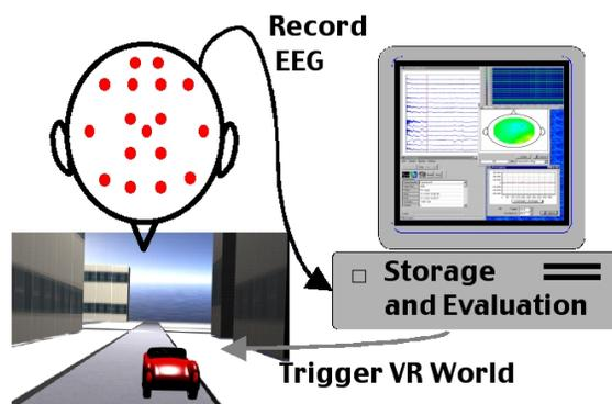
Figure 1: Sketch of low-cost experimental setup, to record EEG/ERPs while driving in a virtual environment.
