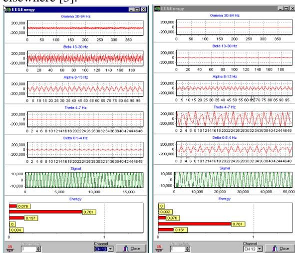
Figure 2: EEG-band decomposition panel. Left for a 20Hz, right for a 5 Hz sinusoidal signal. From top to bottom are  $\gamma$ ,  $\beta$ ,  $\alpha$ ,  $\theta$ , and  $\delta$  components and the original signal over time displayed. The bottom most bar graph shows the energy at any given moment.
