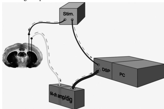
Figure 3. Schematic overview of the electronic set-up. Stimulation is achieved through one microelectrode, while the multisite Niotrode is used to record resulting stimulation patterns from the network.
