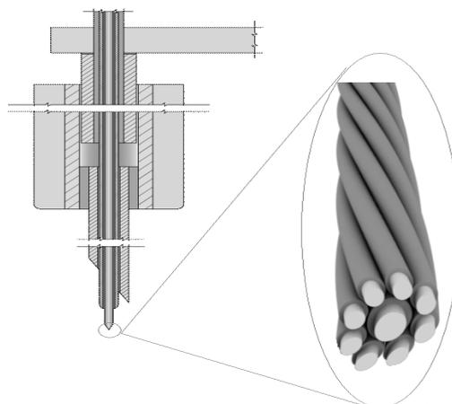
Figure 2: Design sketch of the microwire assembly (right) in a series of concentric guide tubes (left).
