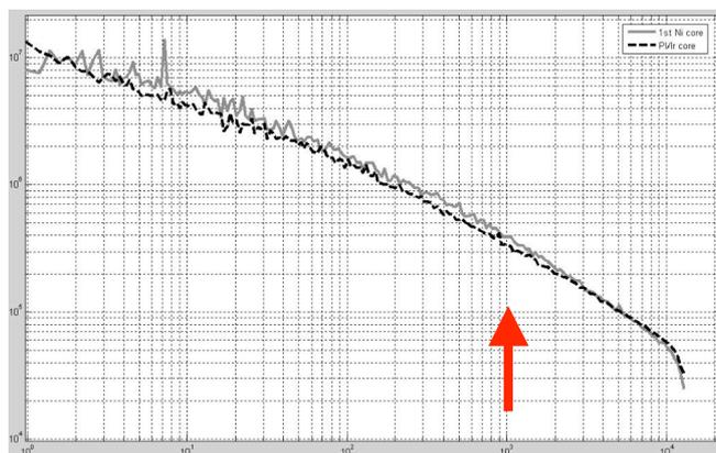
Figure 5: Averaged estimates of impedance spectrum of recording sites Ni1 and the Pt/Ir core of an exemplary Niotrode. Arrow depicts the physiologically relevant impedance at 1kHz.
