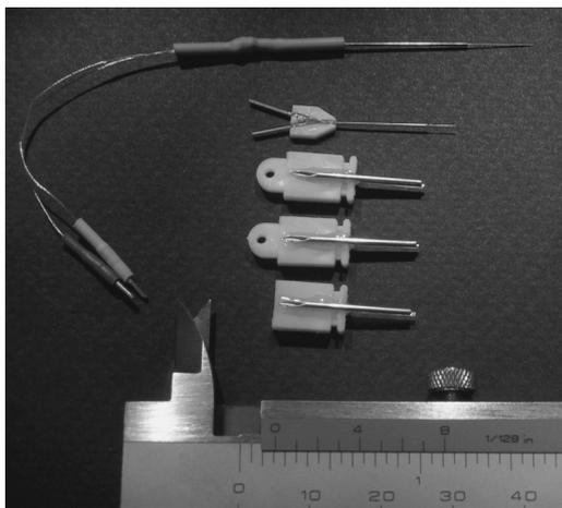
Figure 1: Manufacturing picture of collocated probe stacks. From top: Stimulating electrode, microdialysis probe and different guide tube stacks.
