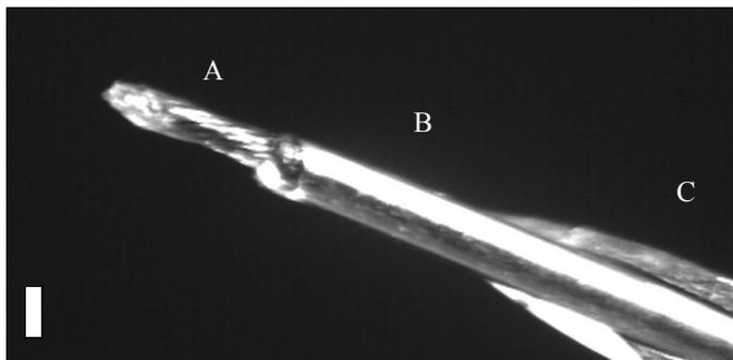
Figure 4. Nine-wire recording electrode: **Niotrode**. Bar depicts ca. 100 $\mu$ m. A is the actual Niotrode, B a 33G stabilizing tube and C the dura penetrating 27G cannula.
