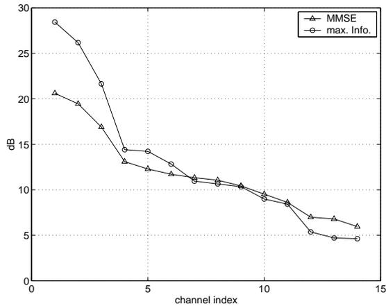
Figure 4: Signal to noise ratios in subchannels at the receiver output.
