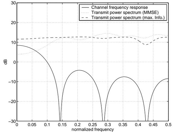
Figure 3: Channel frequency response and transmit power spectra.
