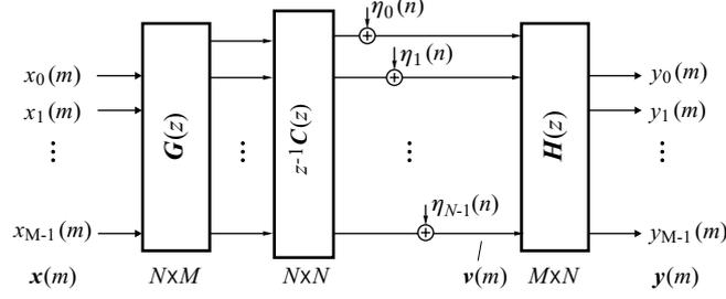
Figure 2: Redundant precoder in polyphase (MIMO) representation.
