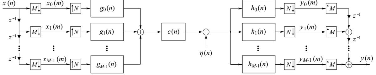
Figure 1: Redundant precoder.
