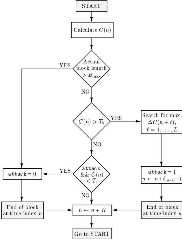
Figure 2: Simplified flowchart of the segmentation algorithm
