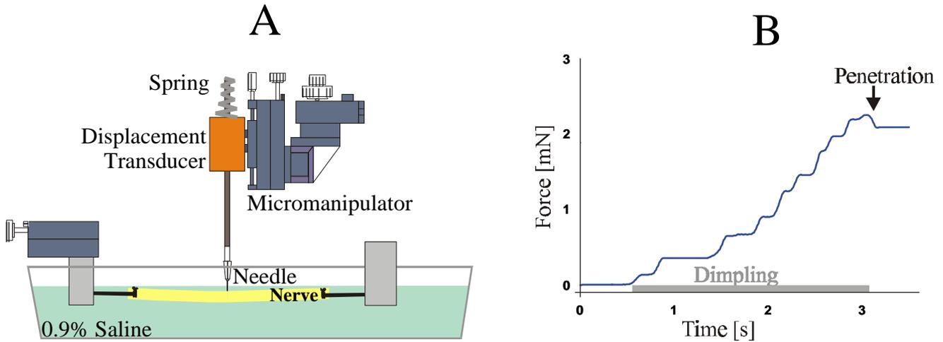
Figure 1. (A) The experimental set-up. During the insertion experiments the peripheral nerve tissue was kept immersed in 0.9% saline solution. The custom build force measurement device consisted of a linear displacement transducer and a steel core moving in its center (B). The force applied to the tungsten needle at contact and insertion plotted as a function of time.
