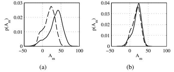
Figure 2: Estimated pdfs for exemplary IIF with clean speech (solid) and with noisy speech (dashed, SNR 10 dB) without PN-processing (a) and with PN-processing (b).
