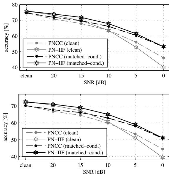
Figure 5: Results for enhanced features under matching (top) and mismatching (bottom) VTL training-test conditions (matched-condition training, black). For comparison, the gray lines indicate the accuracies for the clean-speech training case.
