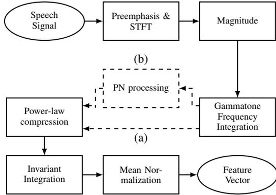
Figure 1: Processing chain for the computation of invariant integration features. (a) originally proposed computation [6]. (b) The combined computation as investigated in this work.
