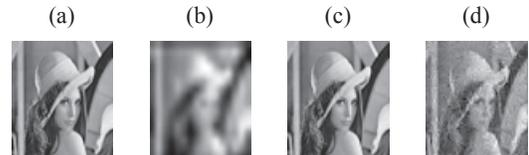
**Fig. 3.** Reconstruction using multi-pixel compressive sensing. (a) Original Image with  $64 \times 64$  pixels. (b) Bilinearly upsampled output of  $16 \times 16$  detectors. (c) Reconstruction using  $M = 20$  measurements with an SNR of 60dB. (d) Reconstruction using  $M = 20$  corrupted measurements with an SNR of 20dB.
