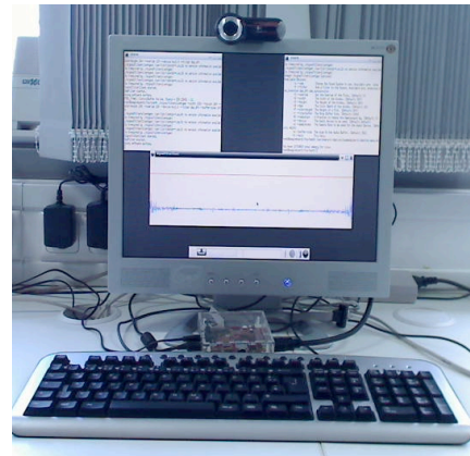
Fig. 2: Physical setup of a BeagleBoard programming environment: The screen in the background shows the DVI output of the boxed BB in the center (arrow), here life audio stream and FFT results.
